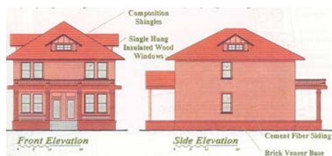
This infill project produced designs compatible with various types of historic architecture. This design is similar to American Foursquare plan houses of the early 20 th century.
