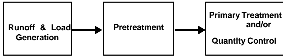
Figure 8.1. Generalized stormwater treatment train.
