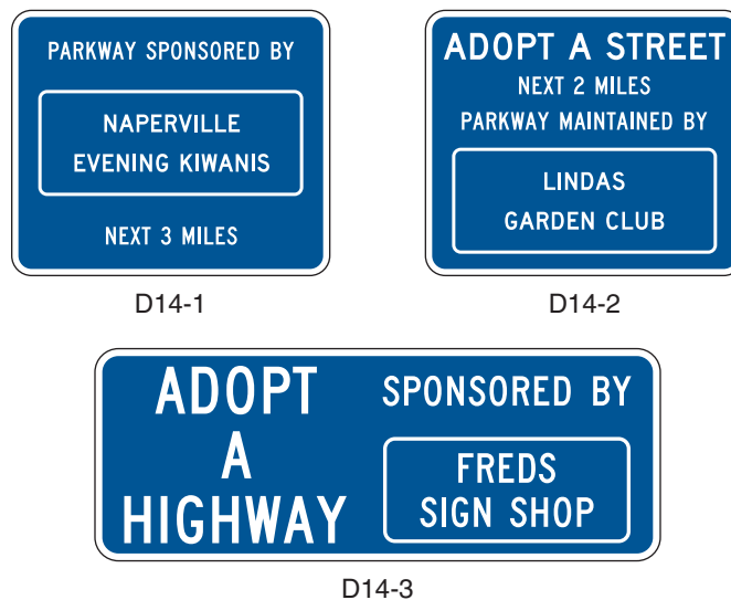
Figure 2H-5. Examples of Acknowledgment Sign Designs
