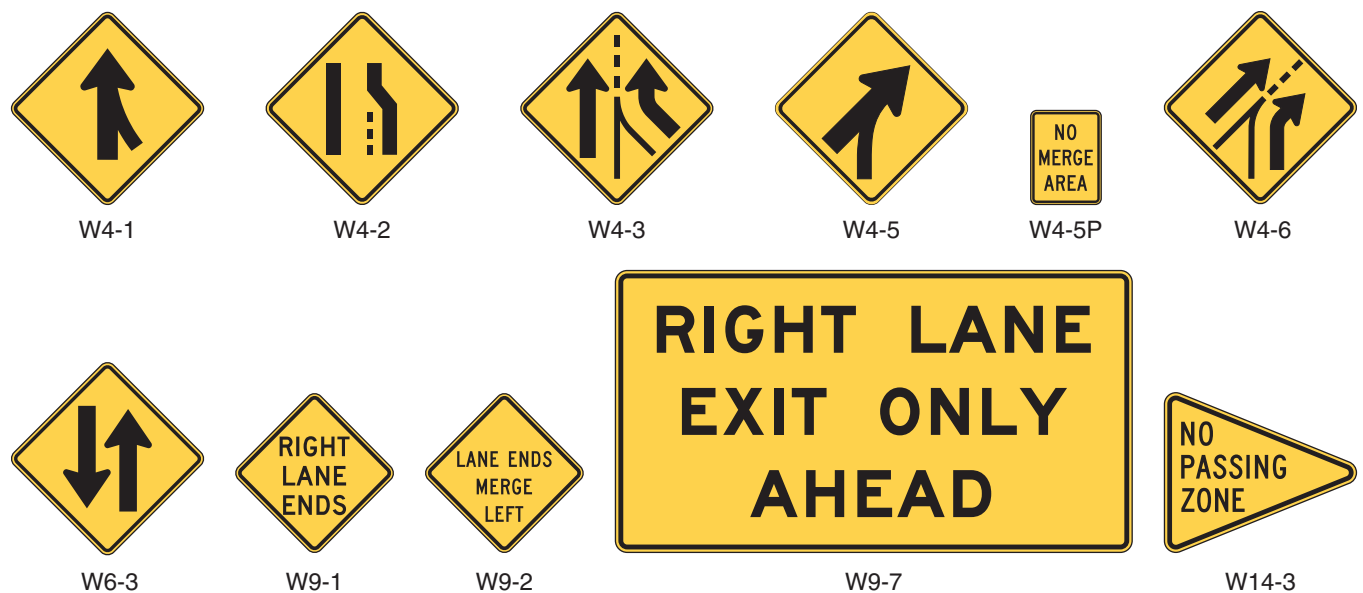
Figure 2C-8. Merging and Passing Signs and Plaques
