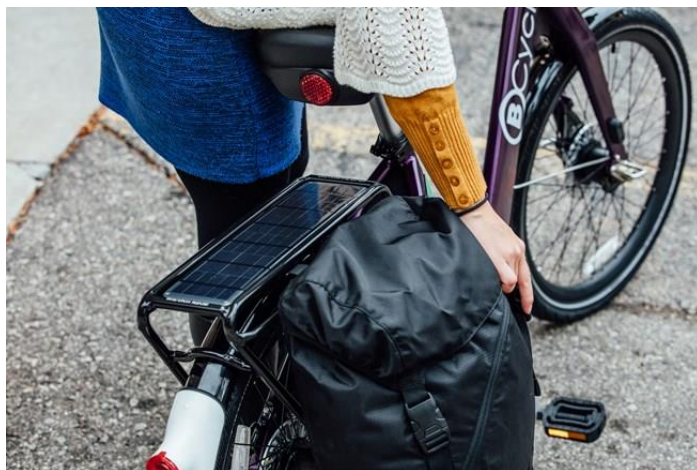
Figure 3. The Dash's solar charging panel on the back rack still provides plenty of space for rear lights
