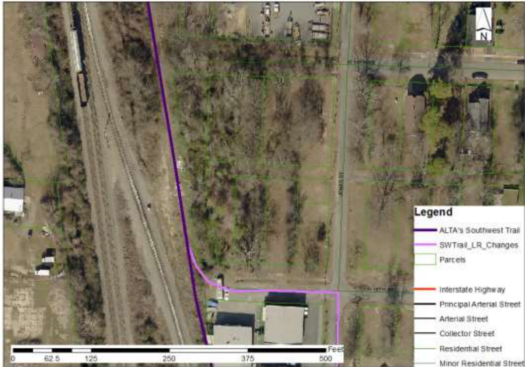
Picture 35. We change ALTA's plan to go onto 18 th St. and then Jones St. because their plan comes too close to active tracks in the next picture. The trail is approximately 52 ft. from active tracks at its closest point here. 18 th St. would be an access point.
