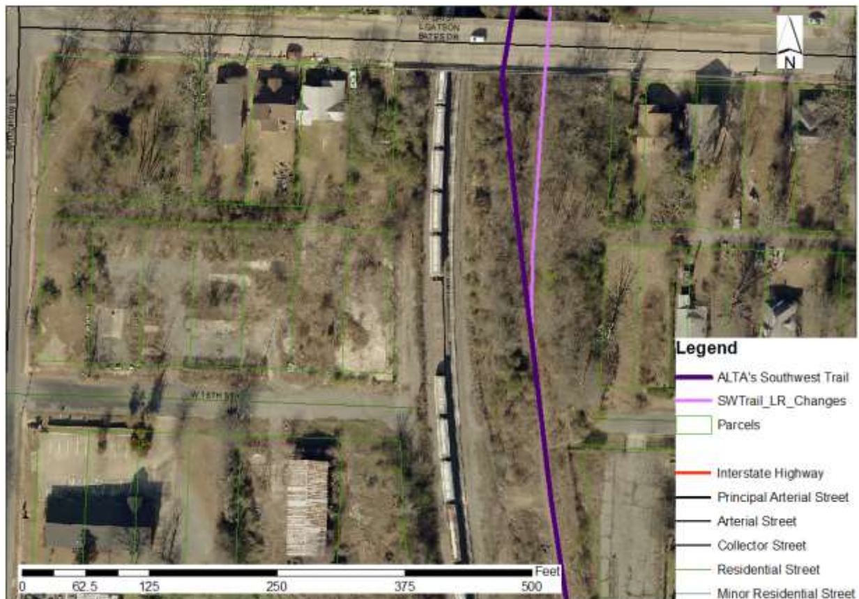
Picture 29. We've altered ALTA's proposed trail to better follow the abandoned line. The trail is approximately 90 ft. from active track at its closest point here. The berm separating the active and abandoned tracks ends around 15 th St. Daisy Bates is a proposed bike route on the Master Bike Plan.
