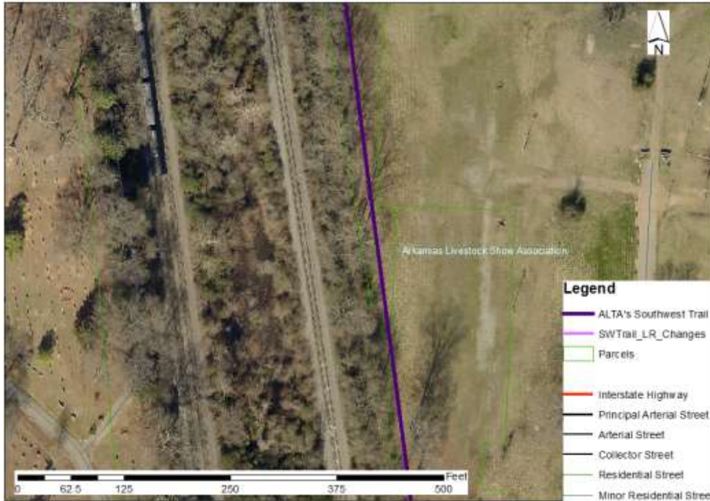
Picture 43. Continued from Picture 41. The trail intersects with a parcel owned by the Arkansas Livestock Show Association. The trail is approximately 82 ft. from active track at its closest point.
