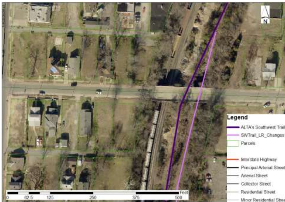
Picture 28. We've altered ALTA's proposed trail to be farther from active tracks and better follow the abandoned line. The trail is approximately 84 ft. from active track at its closest point here and a berm separates active and abandoned tracks.
