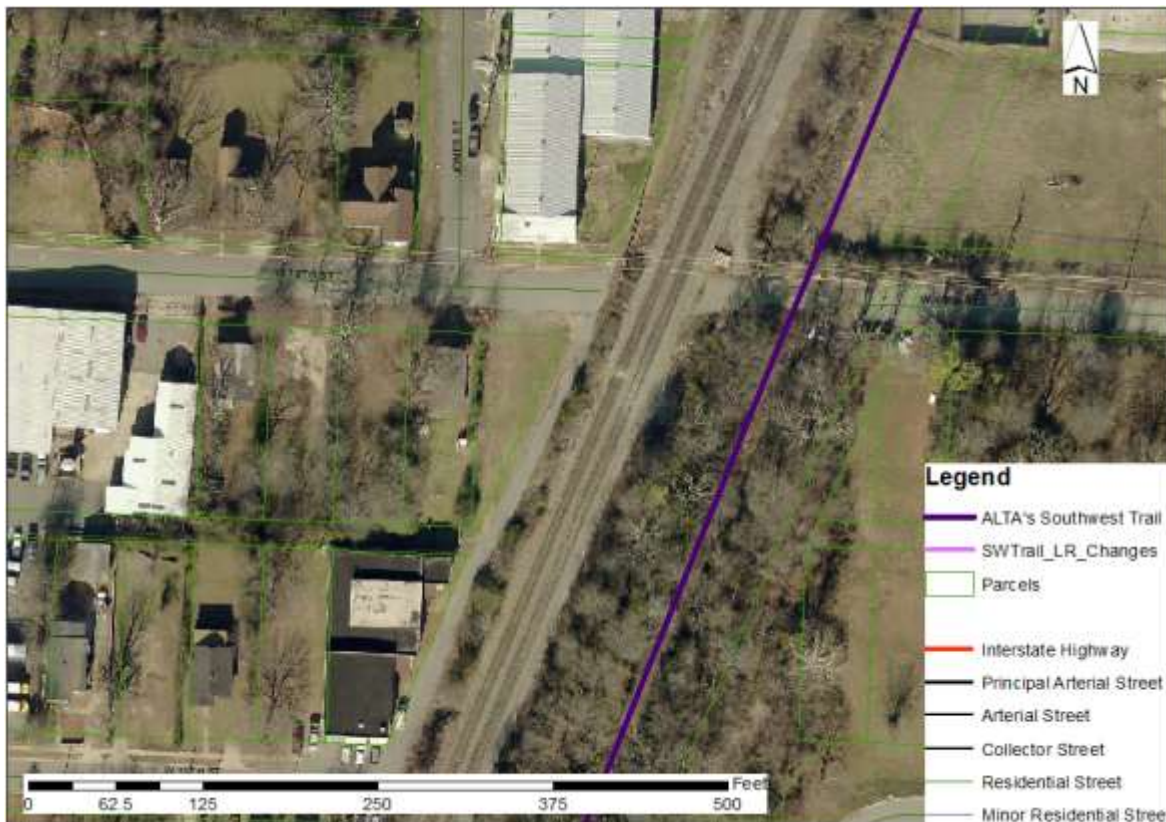
Picture 22. A berm between the active tracks and abandoned tracks starts here and ends around 15 th St. The trail is approximately 82 ft. from active track at its closest point here.
