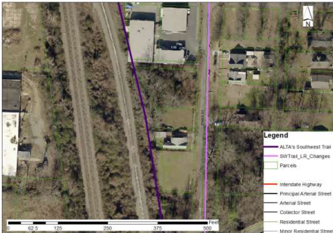
Picture 36. We take the trail onto 18 th St. and Jones St. because the corner of the building comes within 25 ft. of active tracks, leaving little room for a BikePed trail between them.
