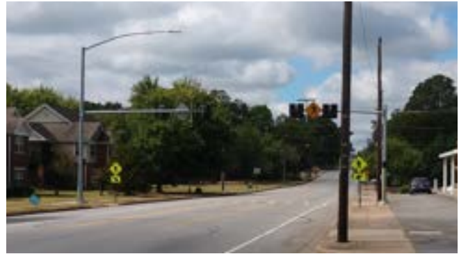
Figure 44: Pedestrian Hybrid Beacons stop automobile traffic for bicyclists and pedestrians wishing to cross a high traffic volume/high speed roadway.
